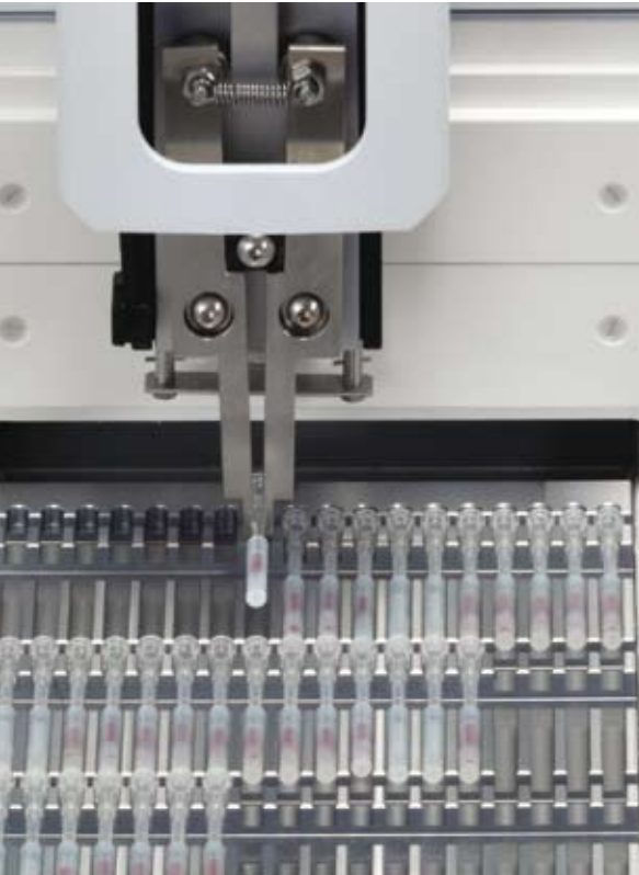
SCAP PLS system robotic gripper tool picks-up sample cartridge...
