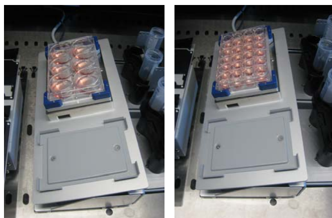
Figure 2 Tilting rack with shaker, 6-well and 24-well plates.
