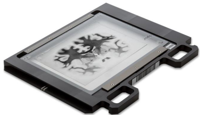
Figure 3. The 5x7" slide of a human brain on Huron's whole-mount slideholder.
